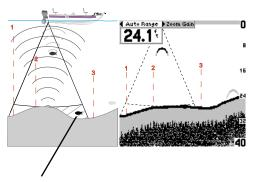
This fish is currently in a Dead Zone and is not detected by the sonar. The fish is in the coverage area of the transducer, but remember the first strong return sets the bottom level. The fish will never be detected since the bottom level will never be set below the fish. The fish on the right side of the display (shown in light grey) will be detected and displayed when the transducer cone passes over the fish.
